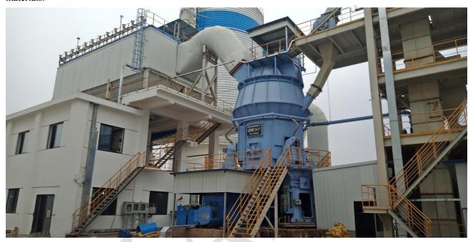
Vertical mill is an equipment that grinds materials by the relative rolling of grinding rollers on the grinding table. The main factors affecting the normal operation of vertical mills are as follows:
